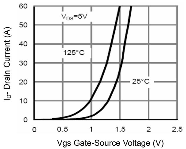
Figure 2 Transfer Characteristics
