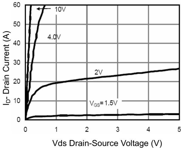
Figure 1 Output Characteristics
