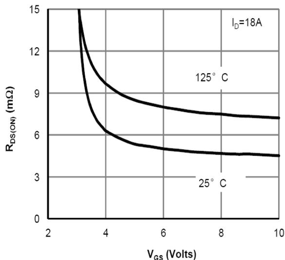
Figure 5: On-Resistance vs. Gate-Source Voltage (Note E)
