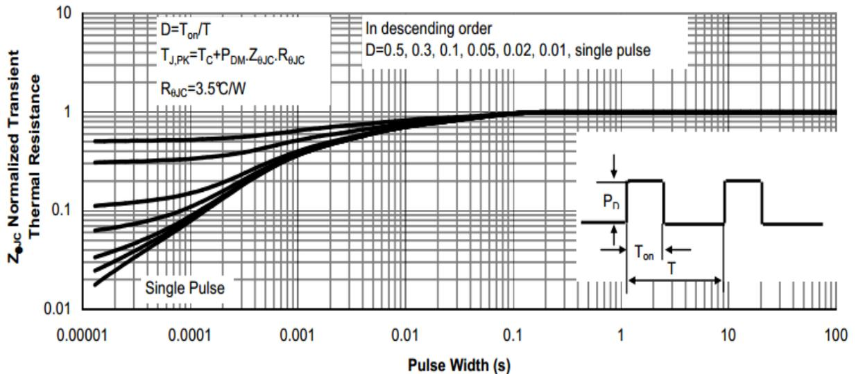
Figure 11: Normalized Maximum Transient Thermal Impedance (Note F)
