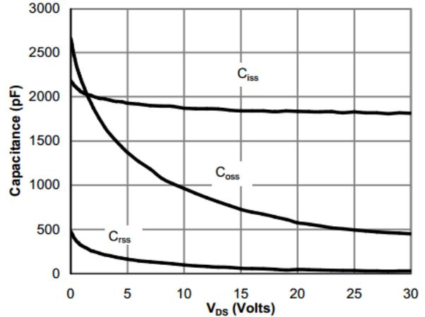
Figure 8: Capacitance Characteristics
