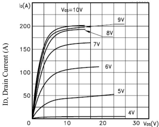
V<sub>DS</sub>, Drain-to-Source Voltage (V)
