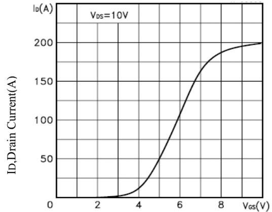
V<sub>GS</sub>, Gate-to-source Voltage (V)
