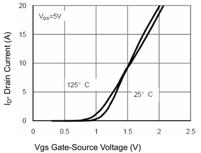
**Figure 2 Transfer Characteristics**
