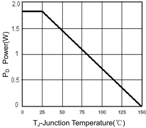
**Figure 1 Power Dissipation VS Junction Temp**
