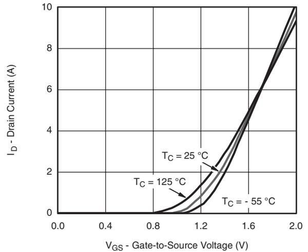
**Figure 4 Transfer Characteristics**
