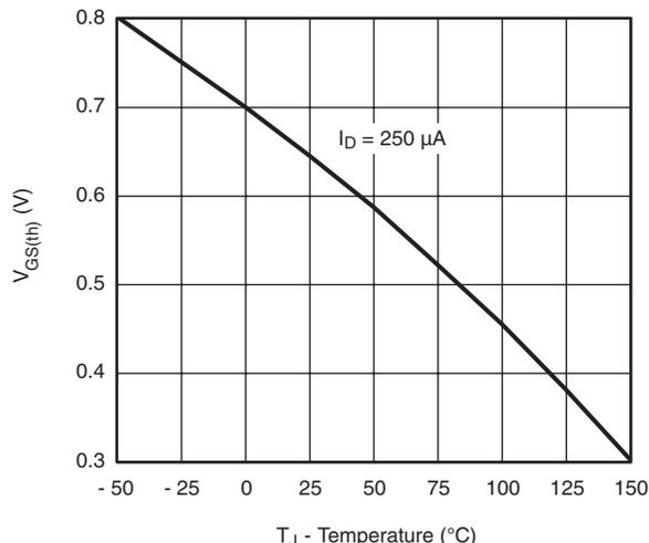
Figure 10 Threshold Voltage
