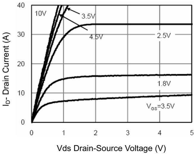
**Figure 1 Output Characteristics**
