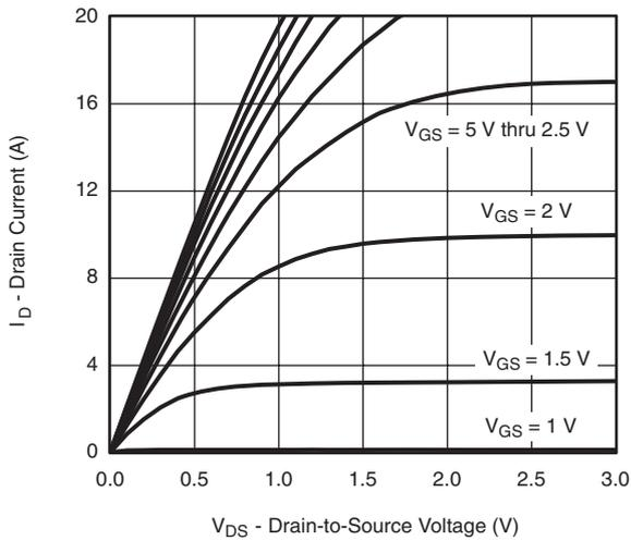
**Figure 3 Output Characteristics**
