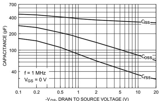
Figure 8. Capacitance Characteristics.
