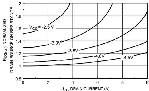
Figure 2. On-Resistance Variation with Drain Current and Gate
