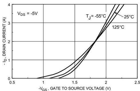
Figure 5. Transfer Characteristics.
