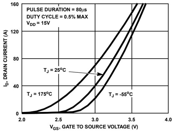
Figure 7. Transfer Characteristics
