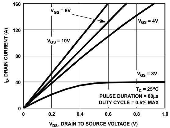
Figure 8. Saturation Characteristics
